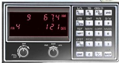
A microprocessor allows navigation to specific fixes or routes
