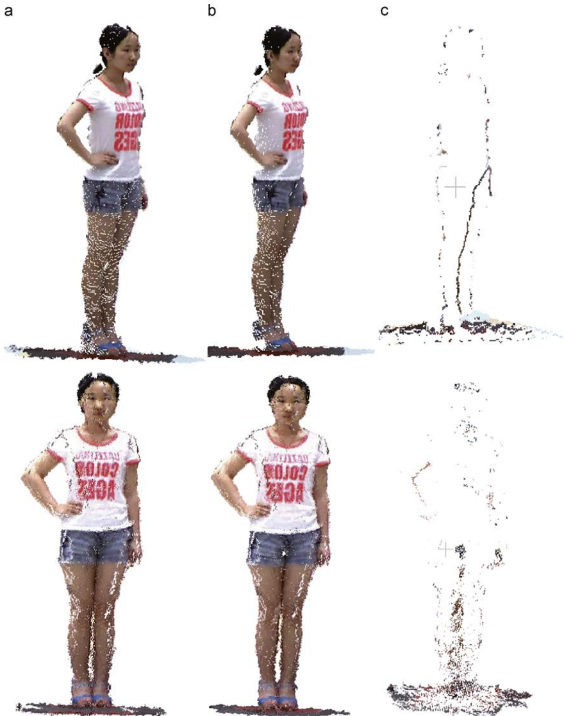
Fig. 3. (a) 3D view without iterative Gaussian filter. (b) 3D view after iterative Gaussian filter. (c) Removed noisy points.
