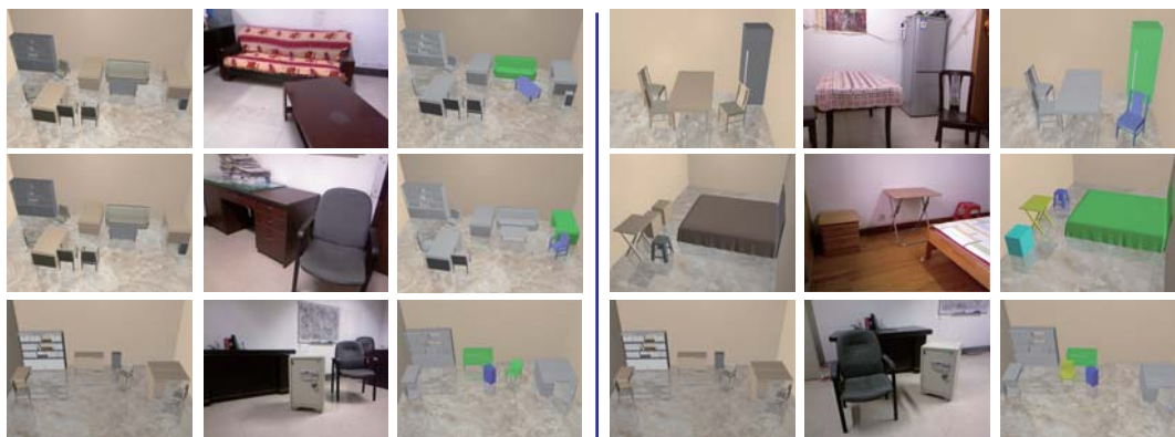
Figure 1: Six groups of scene update results, and comparison between original 3D scene (left) and automatically updated 3D scene (right) by capturing RGBD image (middle) with local variation. The objects in green are seen as static reference, relative to moved objects in other colors.
